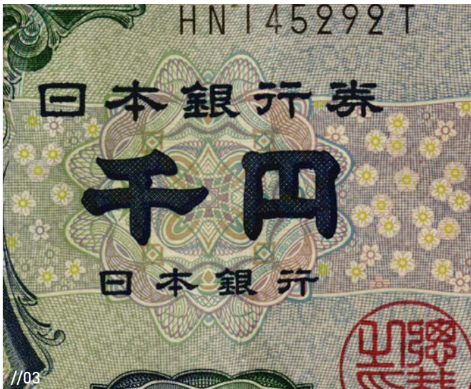
//03 AIT xposure technology: Yen banknote, resolution: 0.05 mm Inspection in real-time at 10 m/s
